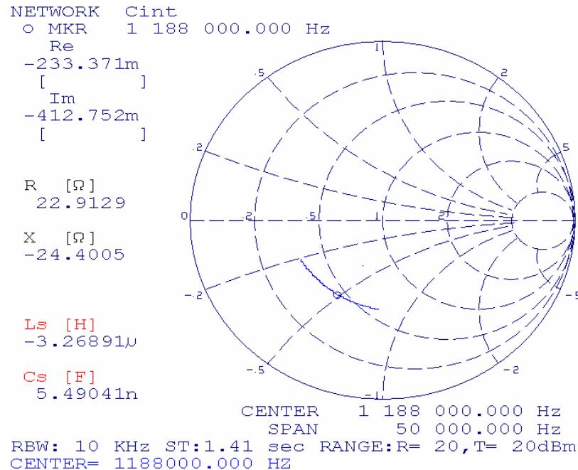
Measuring point MS1C in the drawing
