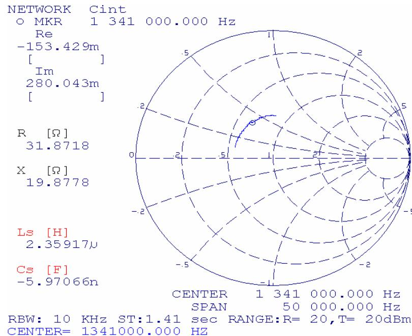
Measuring point MS3C in the drawing
