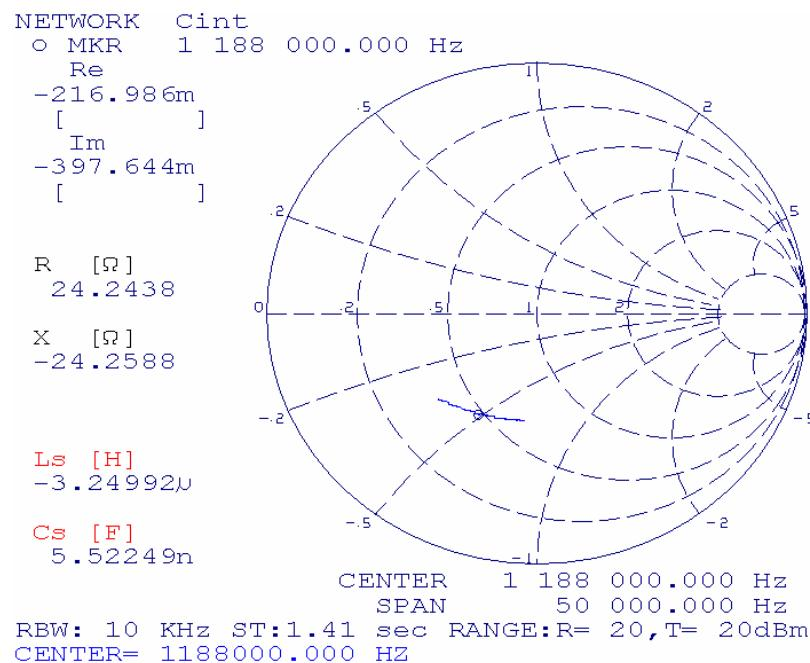
**MW- diplexer Szolnok ( Hungary ) 1188 kHz, 150 kW - 1341 kHz, 150 kW**
